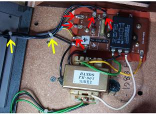
d) Remove the power switch from the old panel by squeezing the ends and pushing it out of the panel. Put this in the new panel with the red printing on the switch to the top (away from the base). Do this by feeding the wires through the hole and pressing the switch into the hole.
