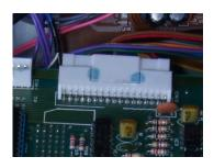
d) Fit the KiwiSix board in the same position and screw in using the four screws that were removed from the KLM-367 in step b. The Kiwisix board in the photo is an early version and will differ slightly.
