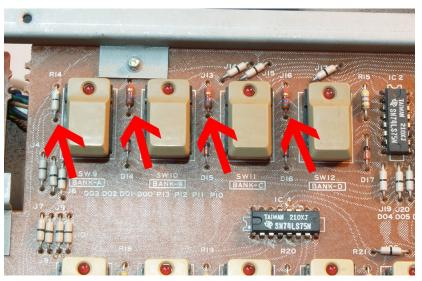
b) Desolder and remove R14, J12, J13 & J16 (red arrows). Use one of the removed jumpers (J12, J13 or J16) to fit a jumper in place of where R14 was and use the 470R resistor in J12. Then fit the two supplied resistors in the J13 & J16 positions (see photo).
