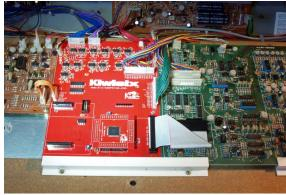
d) Cut the trace between -5v & pin2 and the -5v and pin 4 of IC2. This is done underneath IC2 where the -5v track runs down the center of IC2 and links pin2, pin4 & pin 7. Cut the track neatly between pin 2 and the track and pin 4 and the track leading to pin 7 (arrows in photo shows cuts already made). Pin 7 needs to stay connected to this track so cut carefully. To make sure you have cut correctly make sure there is no short between pin 7 and pins 2 & 4 using a DVM.
