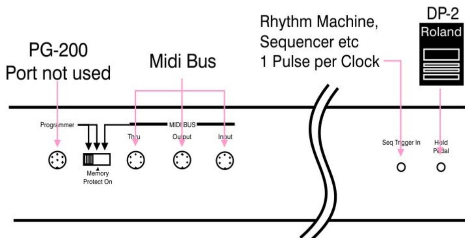
You can adjust the tempo, and start or stop the Sequencer of the JX-3P with the controls on the external unit.
