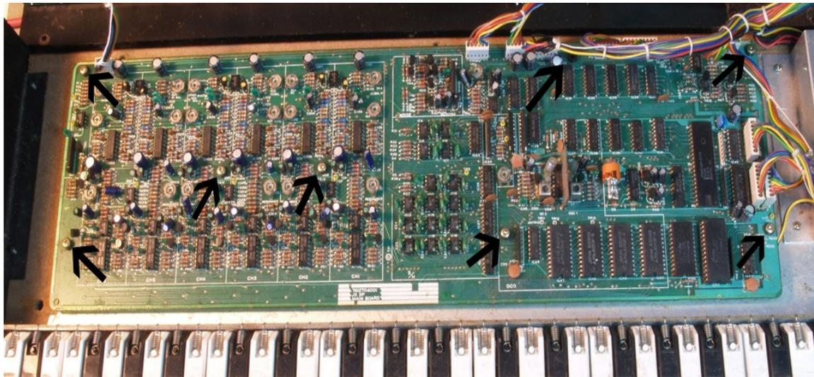
**Photo 1 - Screw Locations in the 3P main board**
