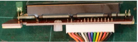
Step 5) The wires going to the front panel need to be moved to make room for the display board. To do this unscrew the two PG200 socket screws so the PG200 socket can be move out from the synth a few centimeters. The wires going to the plugs CN6, CN7 & CN8 need to be moved and put through the PG-200 hole as shown in the photo. These can then be plugged back into CN6, CN7 & CN8 and replace the PG-200 socket using the same screws.
