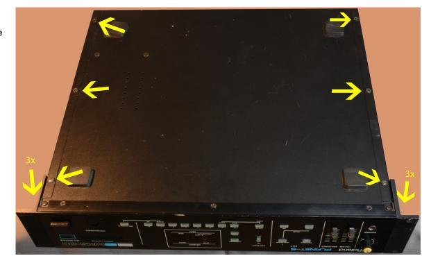
Step 2) Remove the main board. Remove all the cables that are plugged into the board and the 9 screws (marked with yellow arrows in the photo) holding the board into the MKS-30. Lift out the main board. The Blue and Purple arrows are used in the next section for removing the Jack Board.
