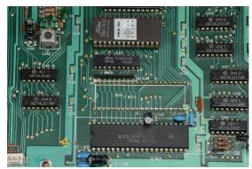
Step 4) Fit the 40pin socket provided into the IC48 area making sure that the notch in the socket is the same orientation as the mark on the board. Check that there are no broken tracks or shorted pins. Bend C148 so that it is a low as possible.
