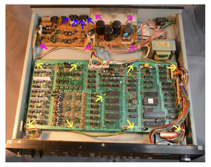
Step 3) Desolder IC48 and C145 and fit the supplied 40 pin IC socket and wires.
