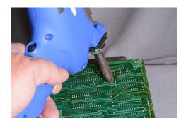
The following IC and parts need to be removed. IC48 (40 pin IC marked 8031 or 8051) and the capacitor right next to it marked C145. These are marked with yellow arrows in the photo. The ROM IC46 is also not required and can be removed if it is in a socket otherwise it can be left as it is ignored by the Kiwi30. The battery is also no longer required and can be removed to prevent any danger of leaking in the future.
