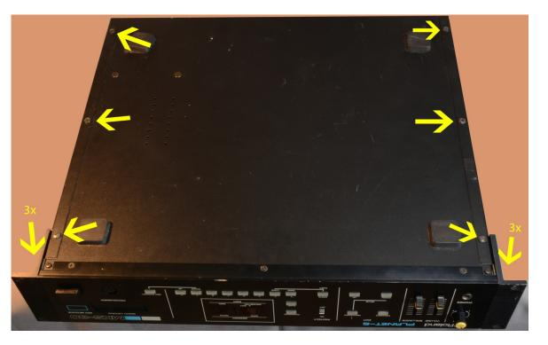
Step 2) Remove the main board. Remove all the cables that are plugged into the board and the 9 screws (marked with yellow arrows in the photo) holding the board into the MKS-30. Lift out the main board. The Blue and Purple arrows are used in the next section for removing the Jack Board.
