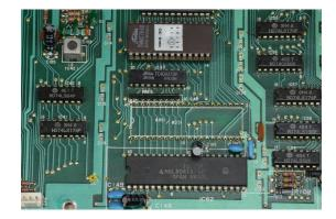
Step 4) Fit the 40pin socket provided into the IC48 area making sure that the notch in the socket is the same orientation as the mark on the board. Check that there are no broken tracks or shorted pins. Bend C148 so that it is a low as possible.
