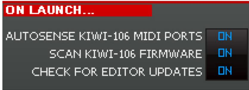
By default the program will AutoSense for the Kiwi-106 MIDI ports then and reconfigure to use these ports for the current session. The program will also scan the Kiwi-106 firmware to be sure it is up-to-date, and it will check with <http://kiwi-106.com> to see if a newer version of the editor (with updated firmware) is available. You can disable any of these startup functions if you wish.
