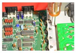
Step 4) Desolder the listed ICs and fit the supplied 40 pin IC socket and links.
